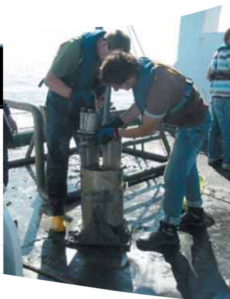
Taking samples to determine the sediment erodibility
