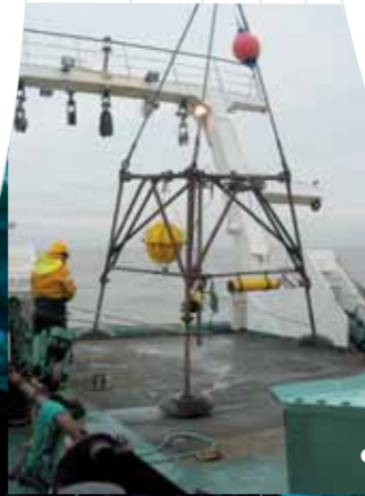
Multisensor tripod for hydrodynamic and sediment transport measurements
